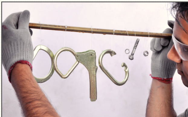
Salt-spray testing for corrosion resistance after zinc plating.
